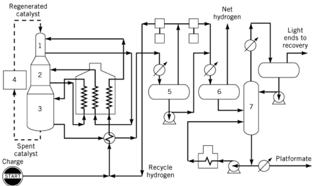
sent through a series of flash separators, 5, 6, and 7, to recover the hydrogen.
